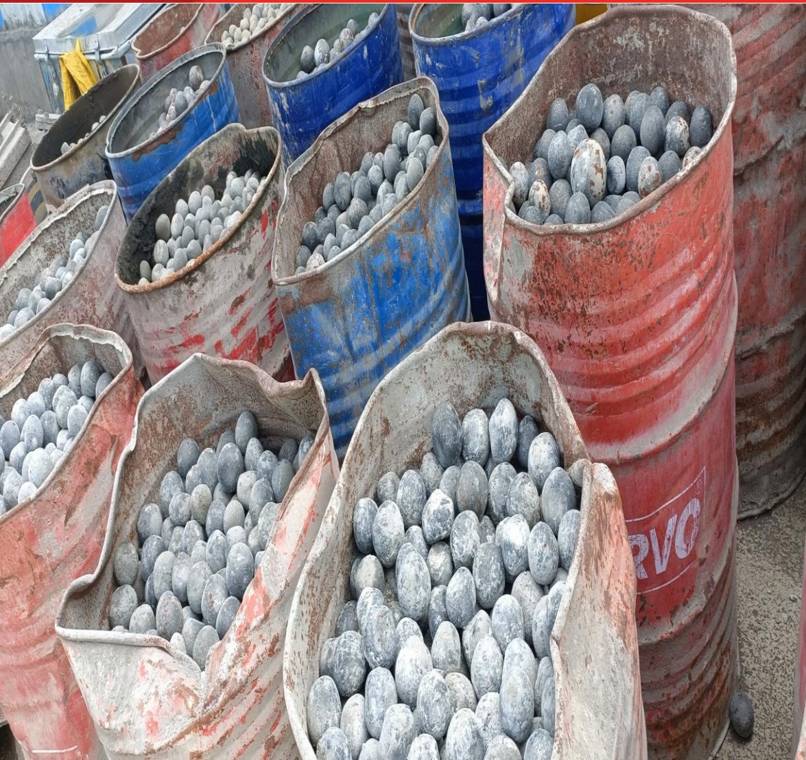
GRINDING MEDIA SCRAP USED (HIGH CHROME)
