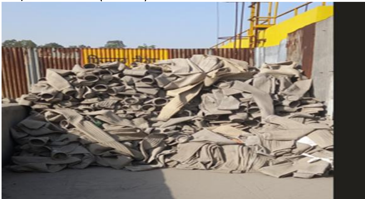
Torn / Used FILTER BAGS ( POLYSTER ) -
