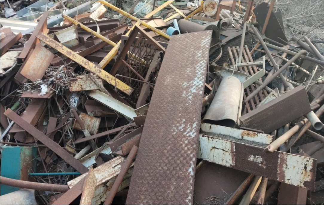
General scrap photos MS heavy with scaling
