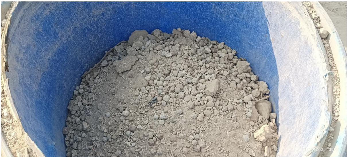
Cement Attached grinding Media
